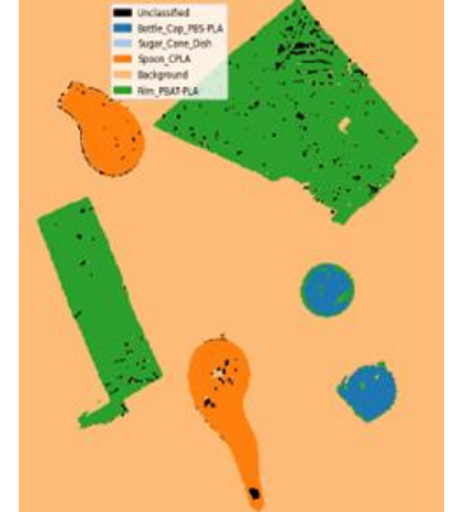
RGB image of the contaminated samples (top) classified contaminated samples from their NIR reflectance (bottom)
