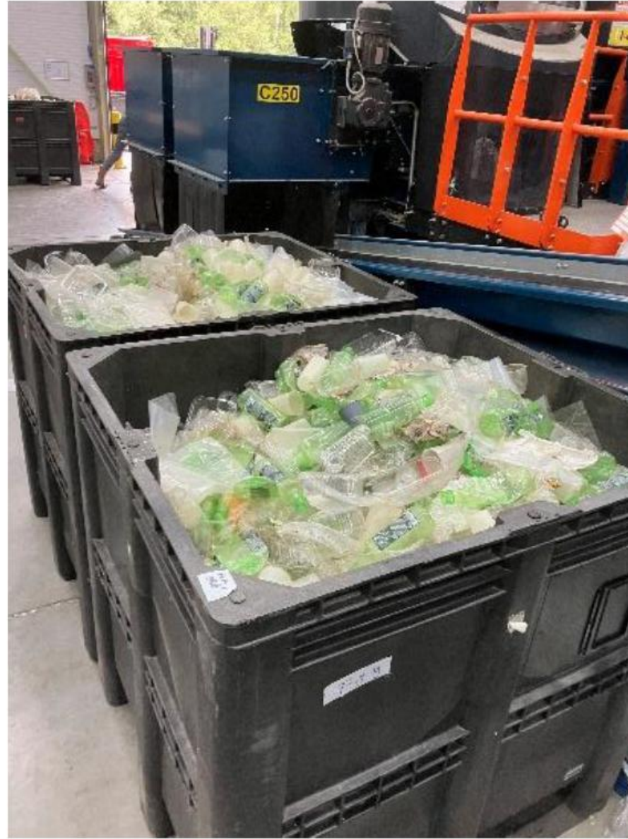
Figure 9 Sorted PLA+PHA fraction, which was subsequently split into separate streams of PLA and PHA
